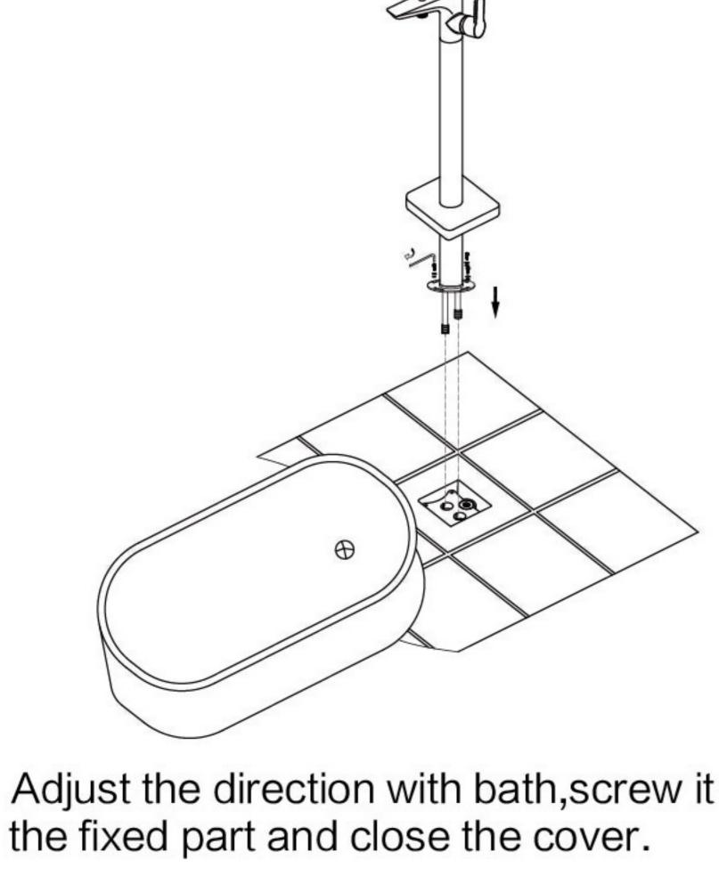
17. Adjust the direction with bath, screw it to
