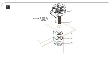
Slide mounting shank(2) through sink from above, add spacer(10) if required, then slide the shank (2) through the rubber washer (3), then through the steel  $\,$ support washer(4). Ensure base is aligned with sink and outlet extends into basin prior to fully tighening mounting nut(5).
